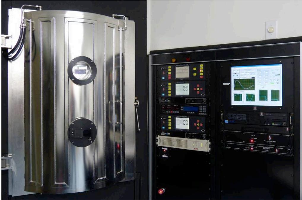
Figure 7 Coating System with SpectraLock IDEM installed
