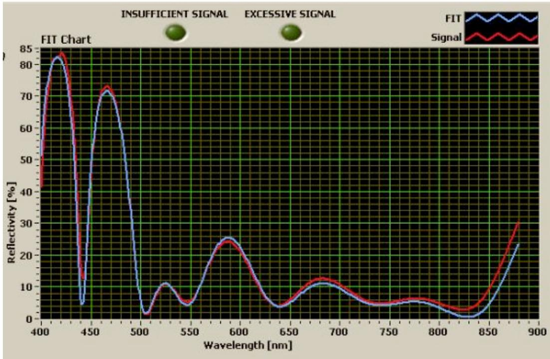
Figure 10 SpectraLock Fit display - Coating Run 4
