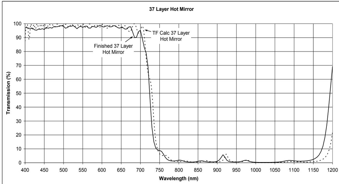
Figure 12 Complex 37 Layer Coating produced with IDEM control
