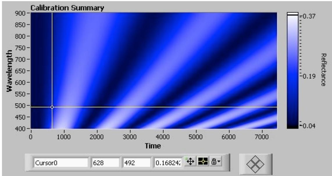
Figure 4 Full Calibration Reflectance vs. Wavelength vs. Time (Thickness)
