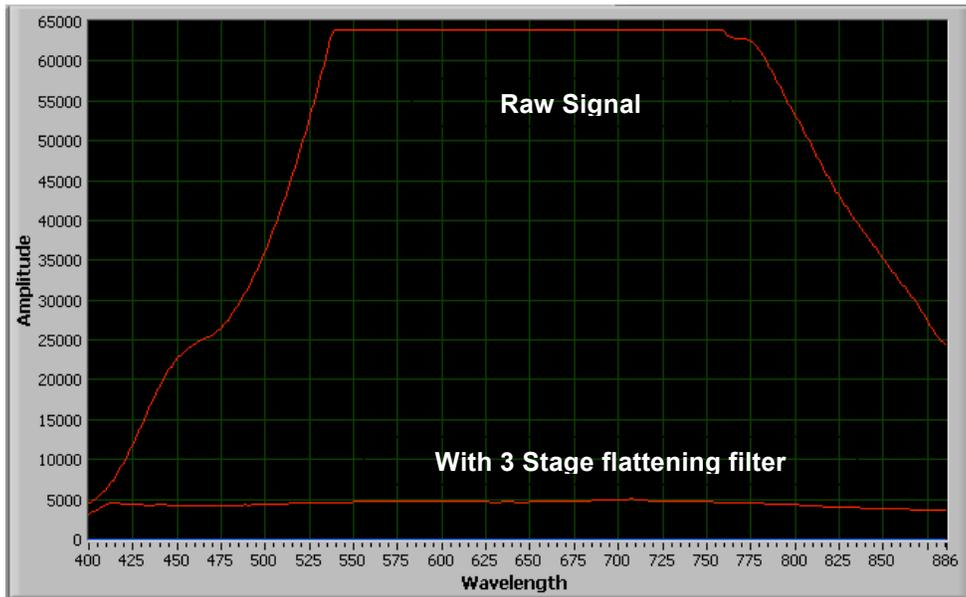
Figure 1 Photodetector Signal with and without Linearization Filter
