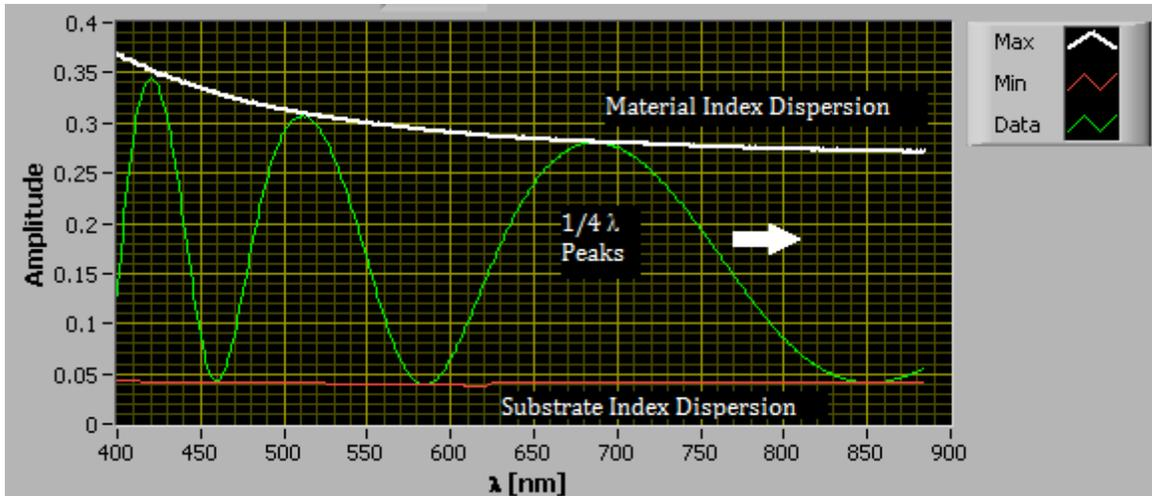
Figure 2 Index dispersion curve obtained during an IDEM calibration run
