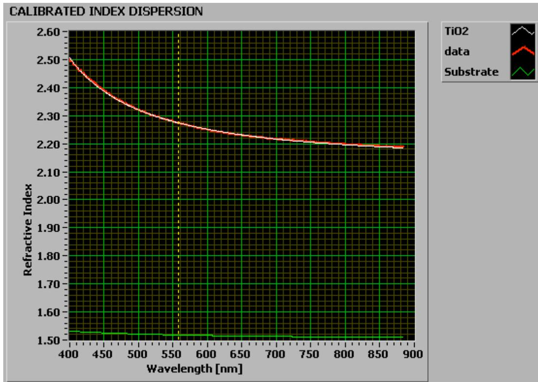
Figure 3 Index calibration curve compared to measured index dispersion
