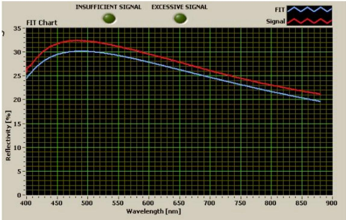
Figure 11 Unrelated Coating - Example of fit needing recalibration
