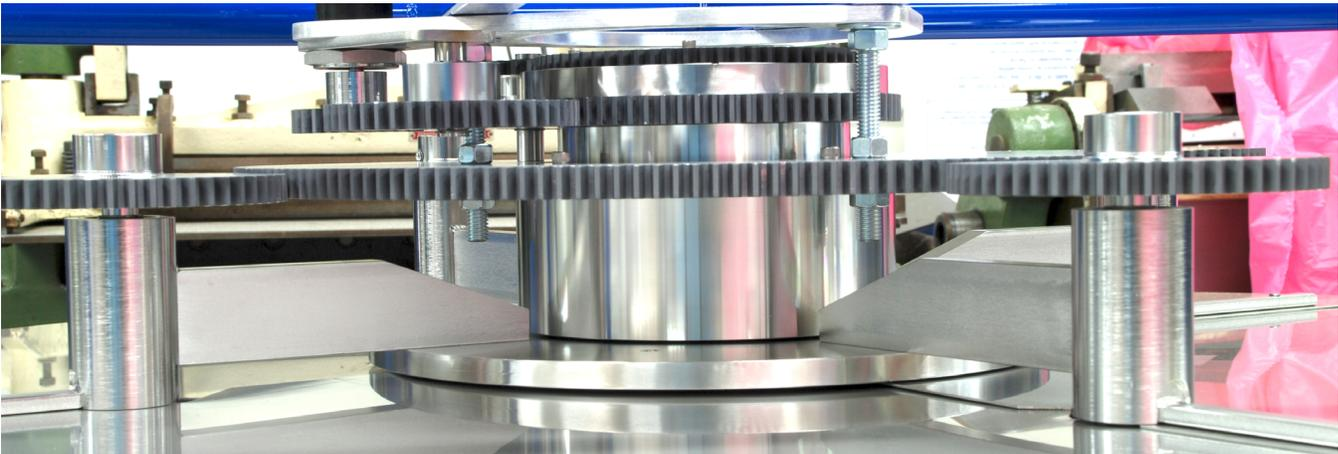
Each gear needs to be coated with a graphite / molybdenum film. This provides the protection they need to operate at up to 300° C in a vacuum. This should be applied as needed to maintain gear life. Also, all threaded parts should be coated to prevent sticking.
