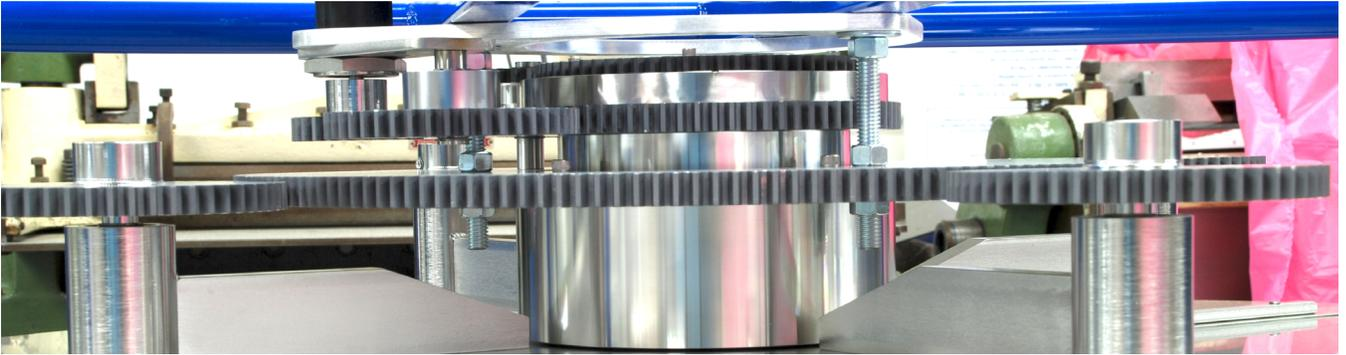
The planetary is mounted on (3) 3/8" dia. threaded rods. Typically we recommend 3/8-24. There should be a minimum of (3) nuts on each rod, one up against the chamber, one up against the top of the main gear and one up against the bottom of the main gear. For added safety and security you can double these up.
