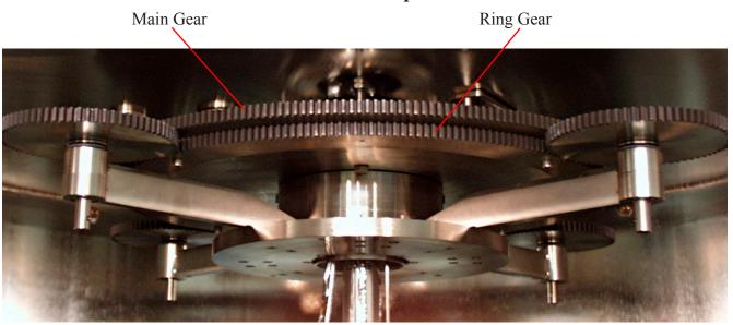
The Ring Gear is included with the PL-481712U and the PL-481714U planetaries. It can be added to a PL-4817U as an upgrade. This allows for the addition of (6) 14 inch or (8) 12 inch planets.
