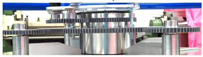
The planetary is mounted on (3) 3/8" dia. threaded rods. Typically we recommend 3/8-24. There should be a minimum of (3) nuts on each rod, one up against the chamber, one up against the top of the main gear and one up against the bottom of the main gear. For added safety and security you can double these up.
