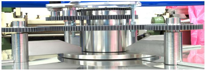
Each gear needs to be coated with a graphite / molybdenum film. This provides the protection they need to operate at up to 300° C in a vacuum. This should be applied as needed to maintain gear life. Also, all threaded parts should be coated to prevent sticking.
